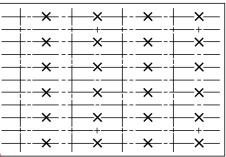
Ceiling grid braced back to structure above - Sliding connection around entire perimeter
