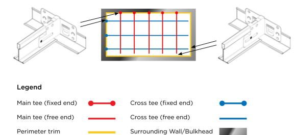
**NOTE:** The building engineer must confirm the two adjacent walls are capable of resisting the line loads of the ceiling.
